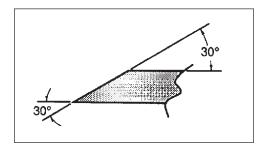
2. DO NOT file the 'gullet' (radius) of the tooth with the flat file. The radius must remain. A sharp corner will lead to a crack and blade failure.
