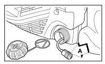
1. Pull Fuel Filter (A) out through gas port, and inspect Fuel Filter.
