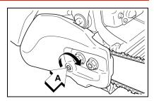
Tighten nuts with the bar nose held up.
