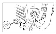
2. If the Oil Filter (a) is dirty, wash it in gasoline or replace it as follows:
