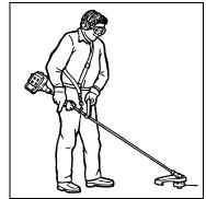
During blade operation, the same fatigue reduction is achieved. Safety to the operator is also enhanced by reducing the possibility of blade contact with the operator's hands and feet by restricting trimmer movement. For more information scan the QR code.
