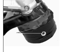
Insert one end of trimmer line into an eyelet, and push line equal distance through trimmer head.
