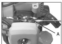
Check idle speed and reset if necessary. If a tachometer is available, idle speed screw (A) should be set to the specifications found on "Specifications" page of this manual. Turn idle screw (A) clockwise to increase idle speed; counter clockwise to decrease idle speed.
