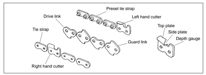
Important points for proper maintenance of saw chain:
