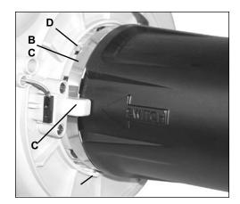
5. Align grooves in discharge elbow with pegs on blower, and slide elbow (D) on to blower. Turn elbow counterclockwise to lock in place. Elbow must angle back toward operator position as shown.
