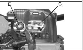
Note: After engine starts, engine decompression button will automatically reset for normal operation.
