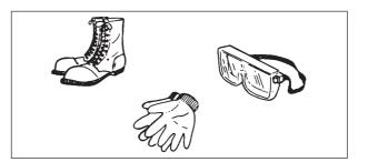
Wear non-slip, heavy-duty work gloves to improve your grip on the engine drill handles. The gloves also help reduce the transmission of machine vibrations to your hands.
