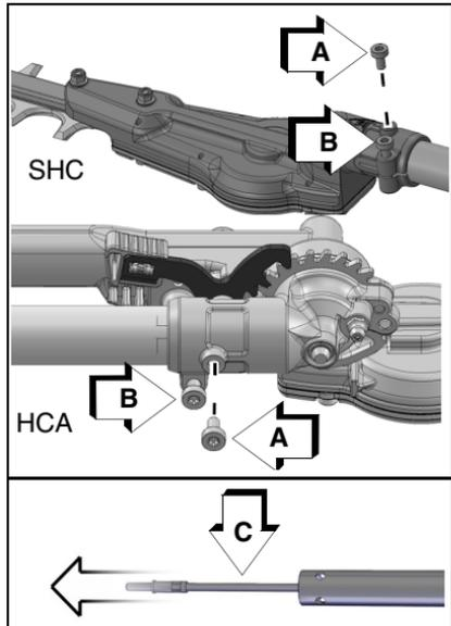
2. Pull the drive shaft (C) from the housing, wipe clean, then apply 15 ml (0.5 oz.) of grease.
