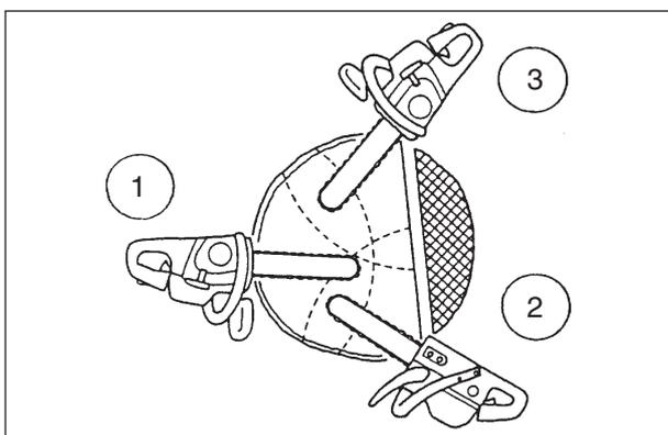
To fell big trees with a diameter exceeding twice the bar length, start the notching cuts from one side and draw the saw through to the other side of the notch.
