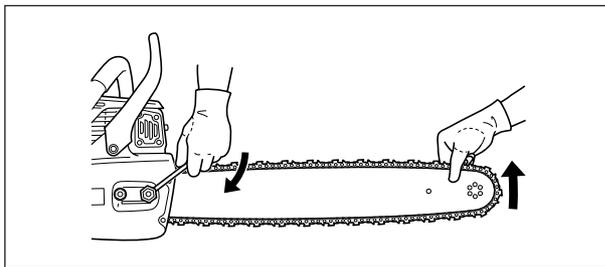
4. Tighten both nuts with the bar nose held up.
