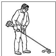
During blade operation, the same fatigue reduction is achieved. Safety to the operator is also enhanced by reducing the possibility of blade contact with the operator's hands and feet by restricting trimmer movement.
