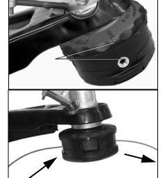
Hold trimmer head while turning knob clockwise to wind line onto spool until about 13 cm (5 in.) of each line remains exposed.
