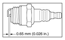
2. Correct the spark gap if it is wider or narrower than the standard gap.
