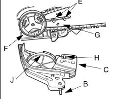
6. Install the sprocket guard (C) over the guide bar studs. Ensure chain tension adjuster pin (H) fits into the guide bar adjuster hole (G), brake band (J) is positioned around clutch drum. Install knob (D) and tighten securely with bar nose held up.
