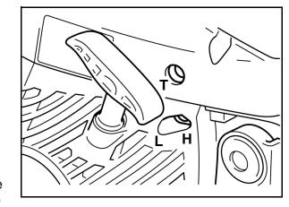
will increase and exhaust emissions will stabilize. Idle speed can be adjusted as required.
