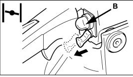
7. Securely hold the chain saw and pull starter handle several times until first starting sound.
