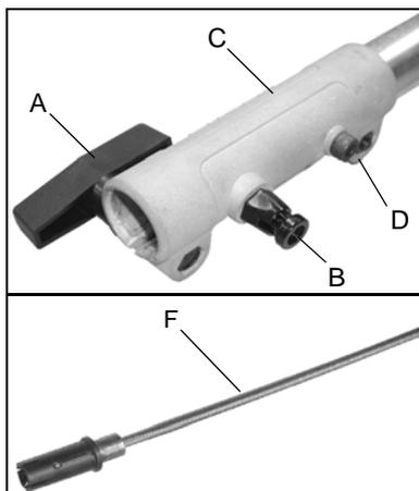
5. Remove upper flex cable (F), wipe clean, and apply a thin coating of 15ml (1/2 oz.) of grease.
