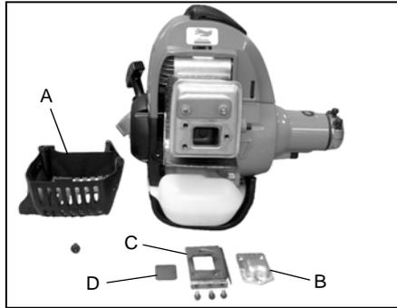
**Note:** When cleaning carbon deposits, be careful not to damage the catalytic element inside muffler.
