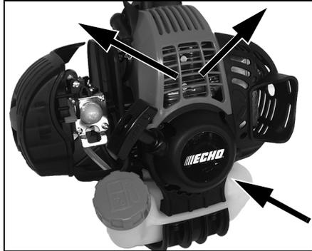
Removal of cooling passage blockages or cleaning of cooling fins is considered “Normal Maintenance.”
