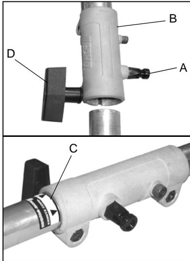
6. Rotate locator pin (A) 1/4 turn clockwise to engage lower shaft hole. Insure locator pin is fully engaged by twisting lower drive shaft. Locator pin should snap flush in coupler. Full engagement will prevent further shaft rotation.
