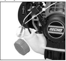
Note: Federal EPA regulations require all model year 2012 and later gasoline powered engines produced for sale in the United States to be equipped with a special low permeation fuel supply hose between the carburetor and fuel tank. When servicing model year 2012 and later equipment, only fuel supply hoses certified by EPA can be used to replace the original equipment supply hose. Fines up to \$37,500 may be enforced for using an uncertified replacement part.
