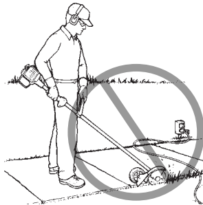
Prohibition - Edger Operation w/Electric Cord on Ground
