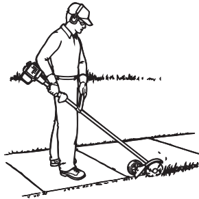
Edger Operator in Operating Position
