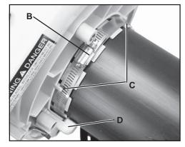
5. Align grooves in discharge elbow with pegs on blower, and slide elbow (D) on to blower. Turn elbow counterclockwise to lock in place. Elbow must angle back toward operator position as shown.
