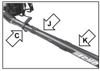
Note: Blower use will eventually loosen pipe connections. Exclusive positive locking system allows pipes to be tightened. If loosening occurs, remove two straight pipes and install according to instructions 8 & 9.
