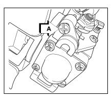
clockwise to increase idle speed; counter clockwise to decrease idle speed.
