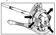
Note: Removal of cooling passage blockages or cleaning of cooling fins is considered "Normal Maintenance." Any failure attributed to lack of maintenance is not warranted.
