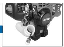
Note: Federal EPA regulations require all model year 2012 and later gasoline powered engines produced for sale in the United States to be equipped with a special low permeation fuel supply hose between the carburetor and fuel tank. When servicing model year 2012 and later equipment, only fuel supply hoses certified by EPA can be used to replace the original equipment supply hose. Fines up to \$37,500 may be enforced for using an un-certified replacement part.
