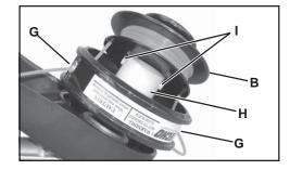
8. Hold drum (A) firmly and turn spool (B) CCW (counterclockwise) until it stops. DO NOT push in on spool when turning.
