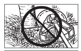
**Use Shoulder/Waist Harness** (P/N 99944200200) Use of the Shoulder/Waist Harness is recommended for **ALL** Trimmer/Brush Cutter use, not just Blade operation. The Shoulder/Waist Harness when used in a trimming operation with nylon line head suspends the trimmer from the operator's shoulder and reduces operator fatigue.
