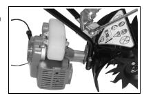
Assemble carriage bolt (A), eye plates (B), lock washer (C), and locknut (D) in front handle mounting holes. DO NOT TIGHTEN BOLTS.
