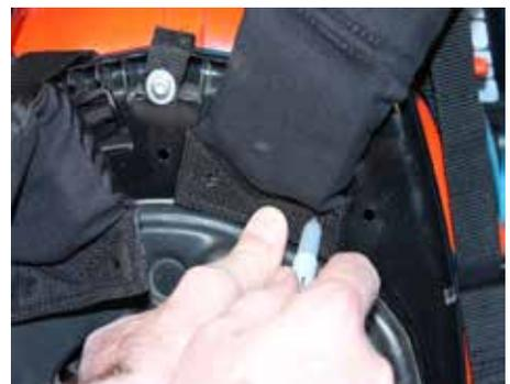
7. Drill holes in frame using a 6mm drill bit.
