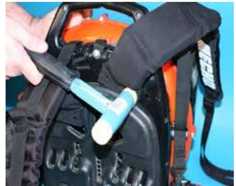
9. Turn lower harness clips sideways, and insert through bottom frame slots.
