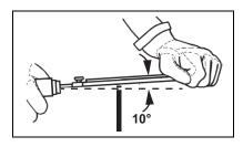
Place the depth gauge tool firmly on guide bar so that depth gauge protrudes. Then file top of depth gauge with the flat file until flat with top of the depth gauge tool.
