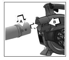
Do not assemble the opposite end of the curved blower pipe to the fan case.
