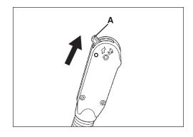
Purge Bulb Pump purge bulb (C) until fuel is visible and flows freely in the clear fuel tank return line. Pump bulb an additional 4 or 5 times.
