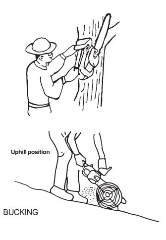
Don't cut with the saw overhead or the bar in a vertical position. If the saw should kick back you may not have good enough control to prevent possible injury.
