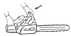
• When the lever is fully pulled toward the operator, brake is released.
