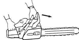
• When the lever is pushed forward, chain brake instantly works to stop the chain.
