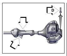
Note: If engine does not start with choke in "RUN" position after 5 pulls, repeat instructions 2 - 5.
