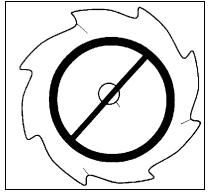
When sharpening a blade, always remove the same amount of materials from each tooth to maintain balance. A blade that is not balanced will cause unsafe handling due to vibration and can result in blade failure.
