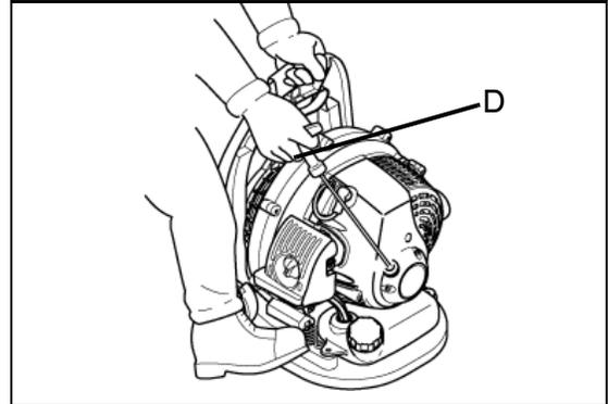
**Stopping Engine**1. *Throttle Position Lever*
