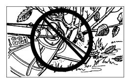
**8 Tooth Weed/Grass Blade** is designed for grass, garden debris and thick weeds. DO NOT use this blade for brush or heavy woody growth, 19 mm (3/4 in.) diameter or larger. SRM-211Series P/N 69600120331
