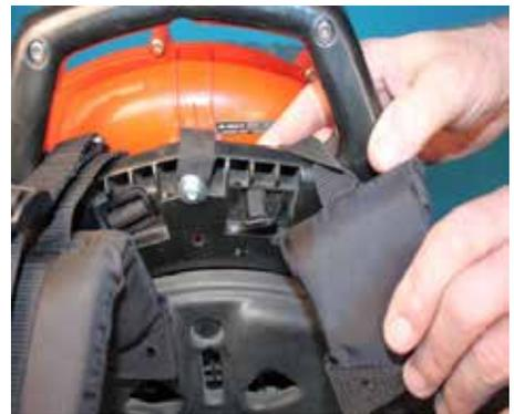
6. Position the harness webbing flush with back pad and at a slight angle as shown. Mark frame through webbing holes with white marker. Repeat for remaining harness.
