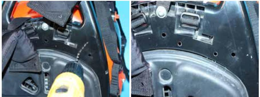
8. Tap new clips in place to secure harness webbing tight against the frame. Repeat steps 5-8 for remaining harness.
