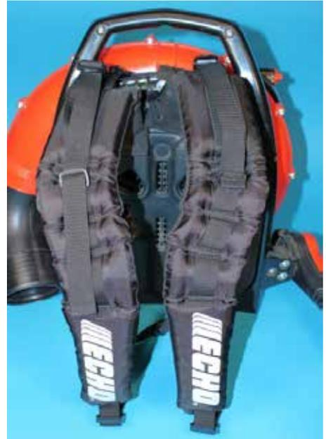
5. Insert upper frame harness clips sideways through upper frame slots and push clips through slots. Rotate clips to retain against the frame wall.
