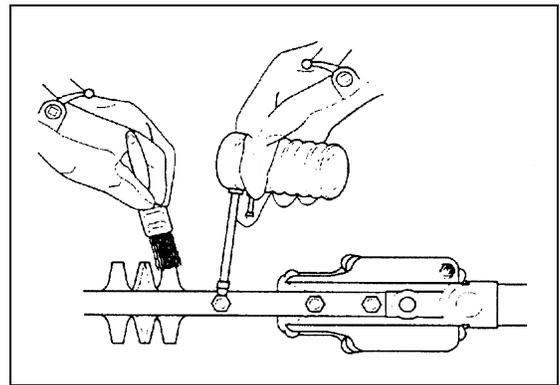
1. Brush loose debris from blade and coat both sides of blade with the 50-50 cleaning mixture.
