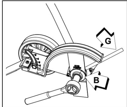
2. Align hole in inner blade adapter (B) with notch in gear housing, and insert locking tool (G) to prevent PTO shaft (C) from rotating.
