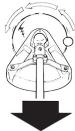
As shown in the illustration, a blade turning counterclockwise will cause the equipment to pull away from the operator if the point of cutting resistance is on the left side of the blade. If the point of cutting resistance is on the right side of the blade, the equipment will push back toward the operator. In both examples, the reactive force is in the opposite direction of blade rotation at the contact point where resistance occurs.
