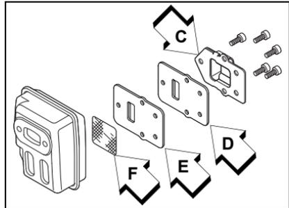
5. Replace screen if it is cracked, plugged, or has holes burned through.
