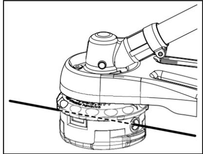
4. Hold trimmer head while turning knob clockwise to wind line onto spool until about 13 cm (5 in.) of each line remains exposed.
