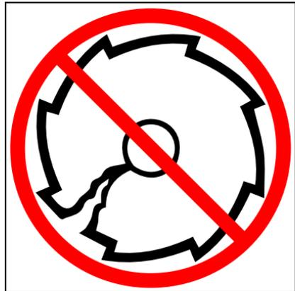
Before sharpening, CLOSELY inspect blade for cracks (look at the bottom of each tooth and the center mounting hole closely), missing teeth and bending. If ANY of these problems are discovered, replace the blade.
