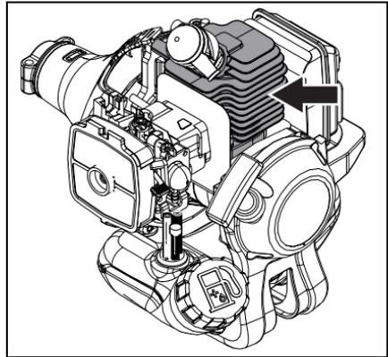
6. Remove grass and leaves from the grid between the recoil starter and fuel tank.
