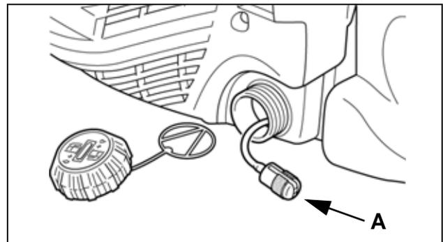
Note: Federal EPA regulations require all model year 2012 and later gasoline powered engines produced for sale in the United States to be equipped with a special low permeation fuel supply hose between the carburetor and fuel tank. When servicing model year 2012 and later equipment, only fuel supply hoses certified by EPA can be used to replace the original equipment supply hose. Fines up to \$37,500 may be enforced for using an un-certified replacement part.
