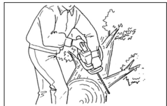
Don't cut with the saw overhead or aligned vertically with your body. If the saw should kickback, you may not have enough control to prevent possible injury.
