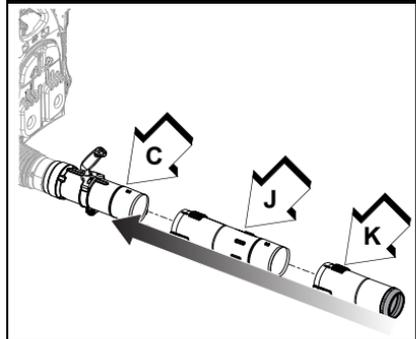
Note: Blower use will eventually loosen pipe connections. Exclusive positive locking system allows pipes to be tightened. If loosening occurs, remove two pipes and install according to steps 8 and 9.
