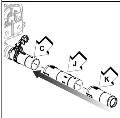
Note: Blower use will eventually loosen pipe connections. Exclusive positive locking system allows pipes to be tightened. If loosening occurs, remove two straight pipes and install according to steps 9 and 10.
