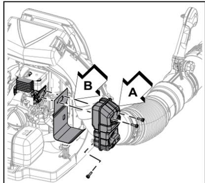
3. Use a wood or plastic scraping tool to clean deposits from cylinder exhaust port.
