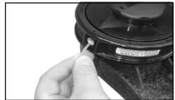
6. Hold drum securely, and turn spool clockwise to wind line onto spool.
