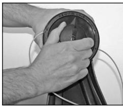
7. Cut remaining line loop to separate into two pieces.
