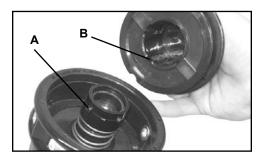
3. Align pegs on inner drive (A) with grooves in spool (B), and install spool onto drum. Do not push down on spool. Turn spool counter clockwise until locking peg clicks into hole in spool (C).
