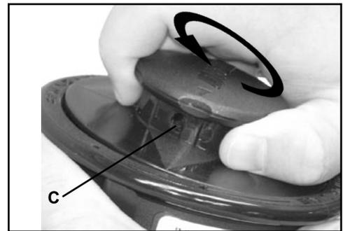
4. Align arrows on spool with marks on drum.
