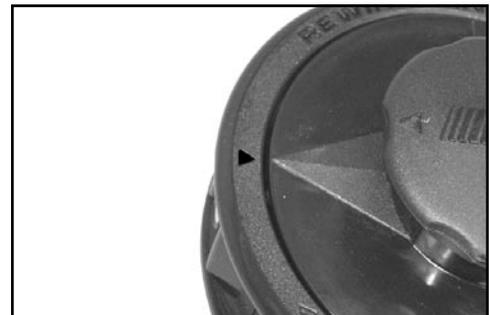
5. Insert two ends of one 24-foot piece of .095 nylon trimmer line into holes on sides of drum.
