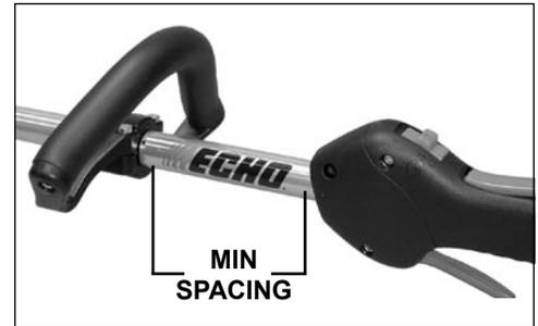
1. Position front handle for comfortable operation and secure screws.
