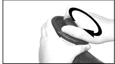
3. Align pegs on inner drive (A) with grooves in spool (B), and install spool onto drum. Do not push down on spool. Turn spool counter clockwise until locking peg clicks into hole in spool (C).
