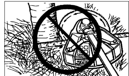
**22 Tooth Clearing Blade** (99944200130) is designed for dense thickets and saplings up to 64 mm (2-1/2 in.) diameter.
