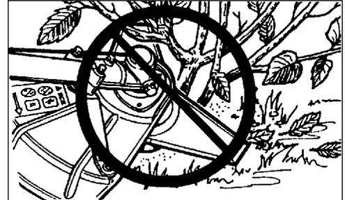
**8 Tooth Weed/Grass Blade** (P/N 69600120331) is designed for grass, garden debris and thick weeds. **DO NOT** use this blade for brush or heavy woody growth, 19 mm (3/4 in.) diameter or larger.
