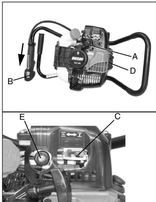
Note: After engine starts, engine decompression button will automatically reset for normal operation.
