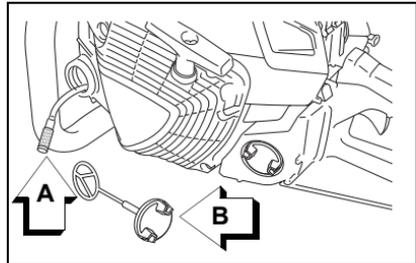
1. Remove the oil cap (B) and pull oil filter (A) out through oil port, and inspect filter.
