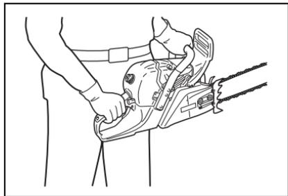
Start the engine, see that it is running properly. Squeeze the trigger to open the throttle wide open and start the cut. If the chain is properly sharpened, the cutting should be relatively effortless. It is not necessary to press down hard to make the saw cut. Pushing the saw too hard will slow the engine and cutting will actually be more difficult.
