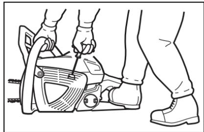
7. Push choke control knob (A) all the way IN (OPEN [↑↓]choke position).
