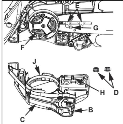
6. Install sprocket guard over guide bar studs. Ensure chain tension adjuster pin (H) fits into the guide bar adjuster hole (G), brake band (J) is positioned around clutch drum (F). Tighten sprocket guard nuts finger tight.
