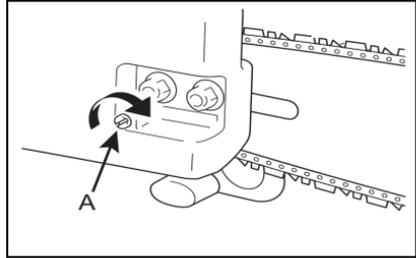
3. Hold the bar nose up, and turn the adjuster toward (+) until chain contacts underside of the bar.
