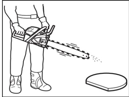
2. Move chain brake lever fully REARWARD to UNLOCK chain brake.
