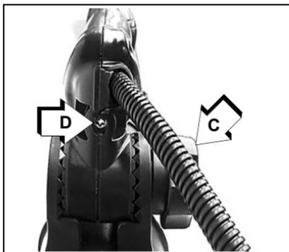
2. Turn adjustment screw until throttle trigger free play is 4 - 6 mm (3/16-1/4 in.).
