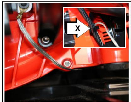
3. Insert the anti-static wire through the flex tube. Leave enough slack in the anti-static wire to allow for full rotation of the elbow.
