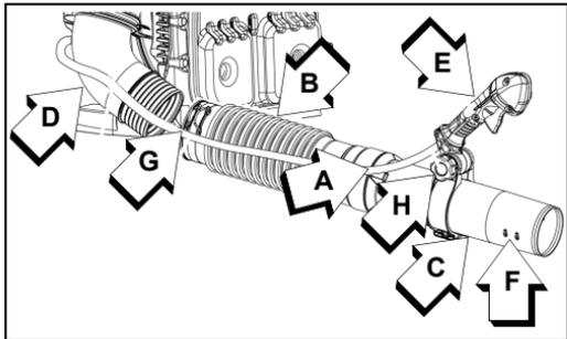
6. Insert the anti-static wire through the swivel pipe (wire will hang freely in pipe).
