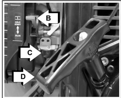
Note: If engine does not start after 5 pulls, use cold start procedures.
