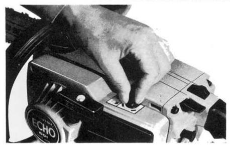
\* For stopping of the engine, release the throttle and pull the switch in the direction of OFF.
