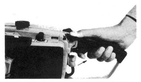
\* For low speed rotation of the engine, adjust it by turning the knob located on the air cleaner. When turned in the direction of H, it will become high speed. When turned in the direction of L, it will become low speed.
