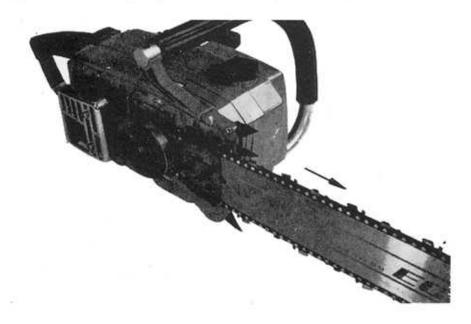
\* To tension the chain, hold up the bar end in one hand and turn the adjusting screw clockwise.
