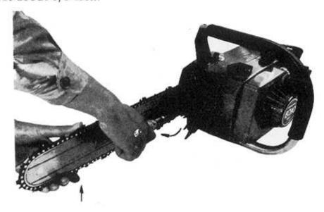
\* Finally tighten up the two nuts with a double-ended wrench while holding the bar end slightly up.
