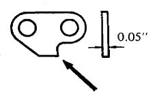
\* The driver link serves to eliminate the sawdust from the bar groove. For this purpose the lower end shall be kept always sharp.
