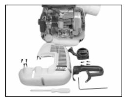
Remove spark arrestor cover (A), gaskets (B) and (C) and spark arrestor screen (D) from muffler. Replace screen if plugged with carbon deposits.
