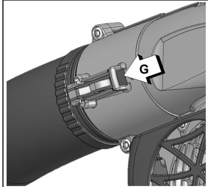
2. Pull pipe out of fan case.
