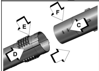
Note: Blower use will eventually loosen pipe connections. Exclusive positive locking system allows pipes to be tightened. If loosening occurs, remove pipe, and reinstall according to instructions 3 and 4.
