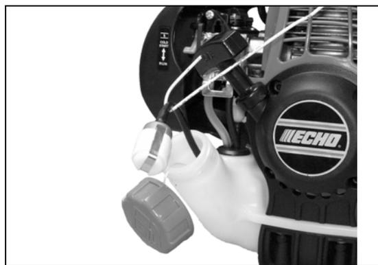
2. Use a hook to pull the fuel line and filter from the tank.
