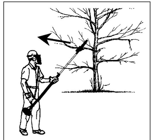
If the saw chain does strike a foreign object, immediately stop the engine, inspect and repair the Power Pruner™ if necessary.
