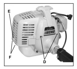
7. Lift the cover from the engine and lay to the front of the trimmer.
