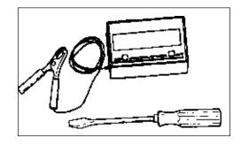
1. Check idle speed and reset if necessary. If a tachometer is available, idle speed screw (A) should be set to the specifications found on page 10 "Specifications" of this manual. Turn idle screw (A) clockwise to increase idle speed; counter clockwise to decrease idle speed.
