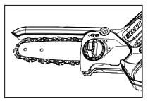
8. Hold the guide bar nose up and turn the chain tension knob (G) clockwise until the chain fits snugly against the underside of the guide bar.
