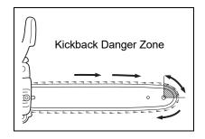
2. Keep a good firm grip on the saw with both hands, the right hand on the rear handle, and the left hand on the front handle, when the engine is running. Use a firm grip with thumbs and fingers encircling the chainsaw handles. A firm grip will help you reduce kickback and maintain control of the saw. Don't let go.
