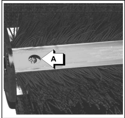
2. Hold 8 mm nut (B) from turning with open end wrench inserted through drum holder cap. Loosen and remove bolt and lock nut with cross head screwdriver through holder access hole (A).
