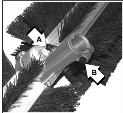
5. Position lower drive shaft (end without serial number decal) into gear housing shaft mount.
