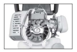
3. Remove bottom left (A) and bottom right (B) hex socket bolts from cylinder cover.
