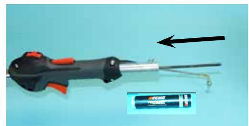
28. Connect the two (2) Ignition Leads between the Control Handle and engine then slide engine onto Main Pipe assembly.
