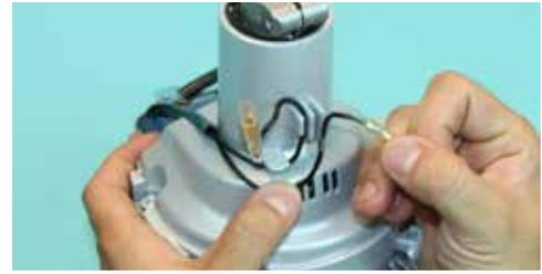
7. Remove upper right and upper left T27 screws from gray Fan Cover and remove Fan Cover from engine.
