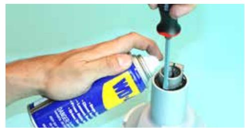
10. Use a flat blade screwdriver to gently pry the Main Pipe Holder from the Fan Cover.
