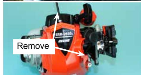
4. Loosen T27 Main Pipe Holder screw and remove Cable Clip.
