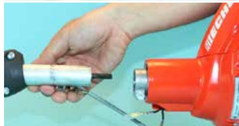
6. Remove two (2) bottom T27 Fan Cover Protector screws, and one (1) drive housing clamping screw. Remove orange outer Fan Cover Protector. Remove ignition wires from gray Fan Cover.
