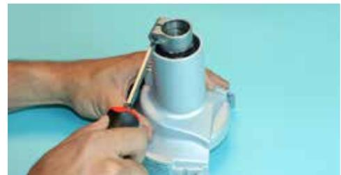
**NOTE:** DO NOT USE EXCESSIVE FORCE otherwise the holder and Fan Cover may be damaged.
