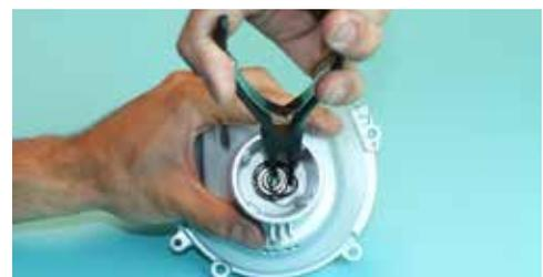
13. Press Clutch Drum from Fan Cover. The press tool diameter should be no more than 11mm or (7/16 inch) in order to clear inner bearing ID.
