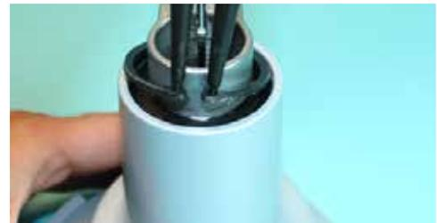
9. Spray WD-40 around top of rubber anti-vibe mount. Use a flat head screwdriver and carefully pry the rubber away from the Fan Cover wall, allowing the WD-40 to penetrate and loosen the seal between the rubber and Fan Cover.
