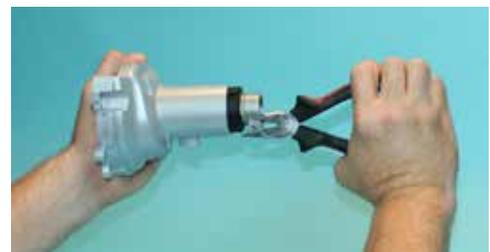
12. Remove the Clutch Drum Snap Ring using external snap ring pliers equipped with .053 tip.
