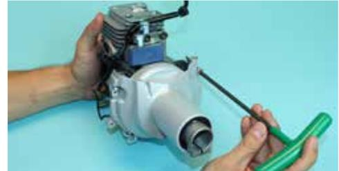
8. Remove Main Pipe Holder retaining ring using external snap ring pliers.
