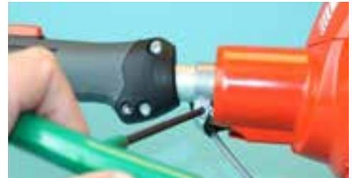
30. Install Throttle Cable end into carburetor Swivel. Install Clip in groove of Swivel to prevent cable end from coming out. Finger tighten Flange Nut.
