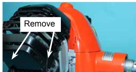
2. Remove Clip holding Throttle Cable on carburetor Swivel. Rotate carburetor rotor to disengage Throttle Cable end from Swivel.
