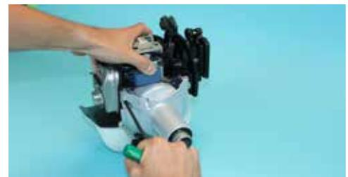
18. Install engine Ignition Leads into protective slots.
