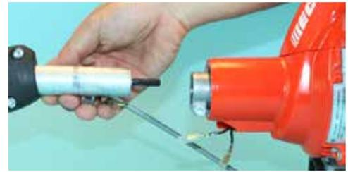
29. Position Cable Clip under Main Pipe then over Throttle Cable and Ignitions Leads. Slide clip tangs under T27 screw head then tighten Main Pipe clamping screw.
