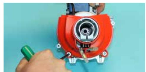
20. Install Engine Cover with two (2) T27 screws using torx driver: rear center, and top left.
