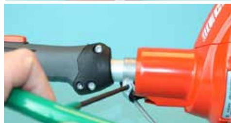
5. Disconnect two (2) Ignition Leads between the Control Handle and engine, then slide engine off Main Pipe assembly.
