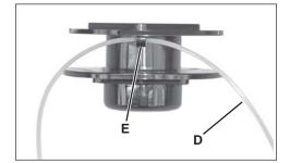
4. Hold spool with the tap knob in your hand and opening toward you. Place index finger between the two lines, and wind line clockwise tightly and evenly.
