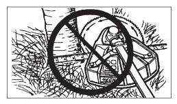
**Use Shoulder/Waist Harness** (P/N 30100052131) Use of the Shoulder/Waist Harness is recommended for **ALL** Trimmer/Brush Cutter use. The Shoulder/Waist Harness suspends the trimmer from the operator's shoulder and reduces operator fatigue.
