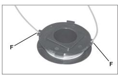
6. Thread line ends through housing eyelets (G) and place spool in housing against spring.
